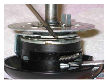
The tab can be pushed up so that it slides on the flat plate and the unit can be rotated slowly. Doing so provides access through 3 holes in the base mount plate to 3 slotted screws.
