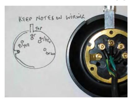
If your plan is to **install a new wiring harness only** and you do not wish to disassemble the control head to access the turn signal switch it is **IMPORTANT** to install the new wires onto the screws one wire at a time.
