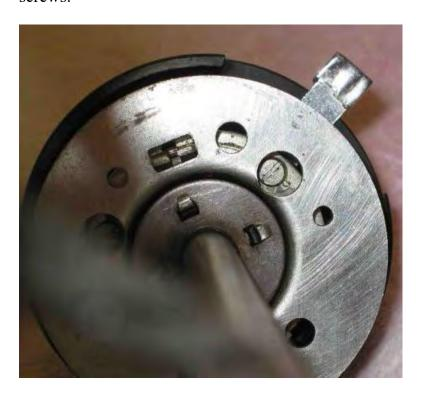
Before removing the three screws, make a note or reference mark of how the two halves of the unit secured by the three screws goes together. Then remove the screws. The correct orientation of the turn signal lever is straight up, but if the two halves are oriented incorrectly, the turn signal lever will be either pointed down, or off to the side.
