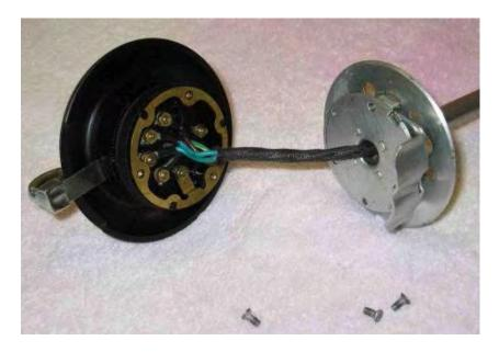
Examine the back of the mounting plate. There are six nuts visible. Three are for the turn signal switch, two are for the horn (one goes through the brass gound ring) and the one without an attached wire is to hold the head and the mounting plate together (It is barely visible in the photo under the wiring sheath). Make a drawing to illustrate the color code and where each of the wires should reconnect to its proper fitting.
