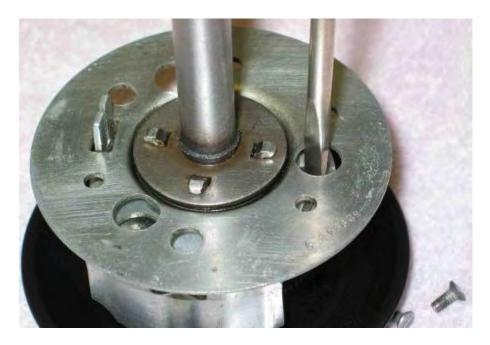
The stator tube, base plate, locating plate, the base mount plate and assorted washers and spring can then be separated from the bakelite mounting plate and head. This assembled unit does not need to be disassembled. It can be pulled off the wires and set aside for assembly later.
