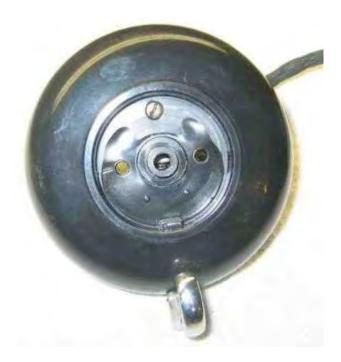
The turn signal lever is attached with one screw to the back of the bakelite mounting plate. Underneath it is a curved wire with a spring on each side of the lever.
