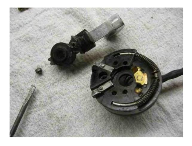
There is another little spring and ball at the bottom of the turn signal lever.
