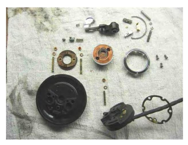
The proper positioning of the two hinges or "triggers" is important. They have angles on the end that fit opposite each other. They need to be placed as seen in the image and drawing for the canceling switch to work. Before reassembly of the complete unit, now is a good time to refinish the bakelite if it is needed.
