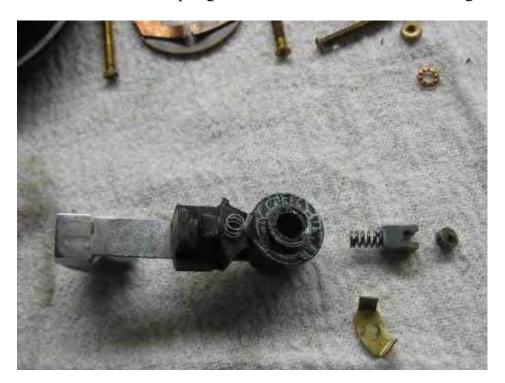
If you carefully remove the single screw to separate the lever from the assembly, the springs and small parts should stay in place. Note how they should be reassembled, then take apart, clean and lubricate with a little lithium grease.
