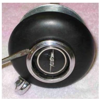
Once the horn button is loosened, the horn spring will be revealed. Its small diameter end faces to the bakelite head. The laminated blades of the horn switch secured by two brass screws also become evident.
