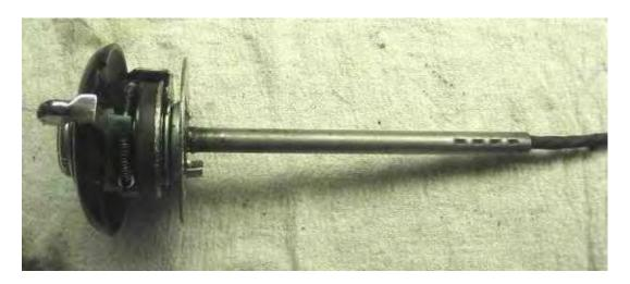
I recommend, based on the comments of others and my own experience, cutting the bullet connectors off the wires, solder the wire or tie the fishing line left in the steering column, to the new wires and slowly pull the new wiring harness through the stator tube and out the end of the steering box. The fit of the harness in the tube is tight so it might be best to tape the wire ends together as they are pulled through.
