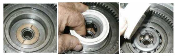
**Dummy Mainshaft:** Several of the procedures require the use of the mainshaft or a suitable fake. If one has the mainshaft out of the gearbox or has a spare, great! The gearbox for this project had already been assembled so I took measurements from the part protruding from the rear of the gearbox and turned a shaft of the same diameter from scrap mild steel. A slot was milled in the shaft and one spline installed to aid later
