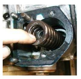
**Installing the Pump Non-Return Valve:** The pump non-return valve is identical the operating valve installed earlier except there is no long spindle. The parts were lubricated and then the ball, plunger and spring were dropped into the hole. The plug with copper washer was then screwed in and tightened.
