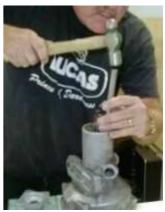
The rear flange was installed again. This time a little gasket sealer was put under the washer to prevent oil leaking along the splines and past the washer. The nut was tightened to  $\sim 100$  foot pounds and then turned on to the next slot for the cotter pin. After everything was together, the shaft was rotated again to make sure it turned smoothly and freely.
