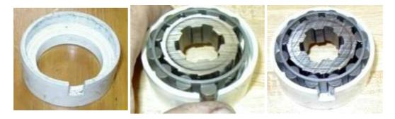
**Installing the unidirectional Clutch:** The rear casting was still mounted to the OD stand. The thrust washer was positioned (left photo), the tool with clutch inside was placed over the recess and the clutch pushed into the recess (center photo), and the tool lifted away (right photo). If one used rubber bands to assemble the clutch, then the procedure is the same and the rubber band would slip off as the clutch was pushed into the recess.
