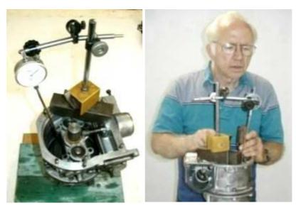
**No End Float!** When the end float was measured with the dial indicator there was none. That was the same result I got using the extra washer method --- but the problems mentioned earlier caused variations of about .010 inch so I didn't know for sure. A problem was suspected because the thrust washer had a grove worn in it. Also, remember that the thrust washer between the sun gear and planet carrier had been destroyed.
