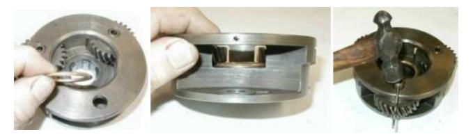
**Installing Epicyclic Gear:** The sun gear can be installed in the planter carrier with the planet gears in various positions. If the gears are not in the correct position, the sun gear shaft will be off center. This would be recognized when it was impossible to pass the mainshaft through the sun gear, the planet
