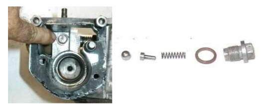
**Removing Pump:** The drain plug and screen filter must be removed to expose the pump.. The photos below were taken after the gearbox had been cleaned up. Much of the oil evaporated from the heat generated when the bearing failed. The outside of the screen was covered by black goo mixed with metal parts. (The later models use a larger plug and the screen is retained by the plug rather than the screw as shown in photos below.)
