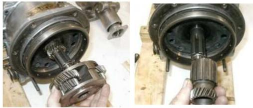
**Removing Main Casting:** The nuts and lock washers from the two bottom studs were removed first. Next, the nuts on the two top studs were loosened; these nuts can't be removed until the main casting is
