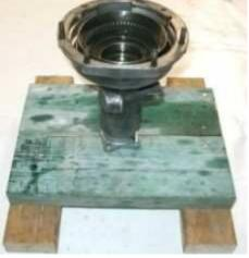
**Annulus End Float:** The annulus end float was measured before the rear casting was disassembled. The end float is adjusted by changing the adjusting washer between the rear bearing and a shoulder on the annulus shaft. If the end float is within spec before disassembly, then it should be within spec even if new bearings are installed because the bearings are made to a very close tolerance.
