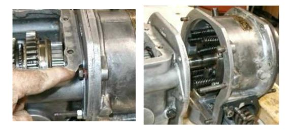
Adaptor: Before leaving the gearbox the adaptor plate surface that mates with the main casting was cleaned and a straightedge used to check to see if it was bent or bowed. If the OD had been previously forced onto the adaptor by tightening the nuts on the studs it is possible that the adaptor is distorted. This will lead to leaks. A severely bent or distorted adaptor can't be used. There have been reports of some success filling minor low spots with epoxy based fillers. The adaptor plate was OK.
