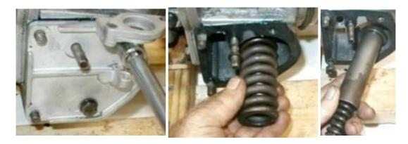
The speedometer bearing & pinion were removed next. This need be removed only if one plans to disassemble the rear casting to replace the two rear bearings. The retaining bolt was removed first, and then the nut from the end of an old speedometer cable was screwed onto the speedometer bearing and a large screwdriver was then used to pry against the lip of the speedometer nut to remove the bearing (left photo below). The parts in right photo were bagged together.
