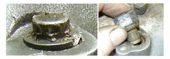
The operating valve components are shown below. The plug and copper washer are new replacements.
