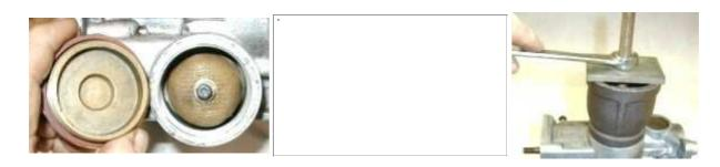
The extracted pump body is shown on the left and with the piston and spring on the right. The hole in the side of the pump body is the seat for the non-return valve ball. The pump components were examined for signs of wear and the valve seat for nicks. The free length of the spring was measured and found to exceed the 2 inch minimum spec.
