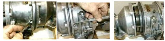
After the rear casting was removed, the planet carrier with planet gears and then the sun gear were removed as shown below. The planet carrier was cleaned and the bearings in each planet gear were tested by rotating the gears. All three gears rotated smoothly and there seemed to be no play in the bearings. It was decided that the planet bearings would not be replaced so it was not necessary to disassemble the planet carrier further.
